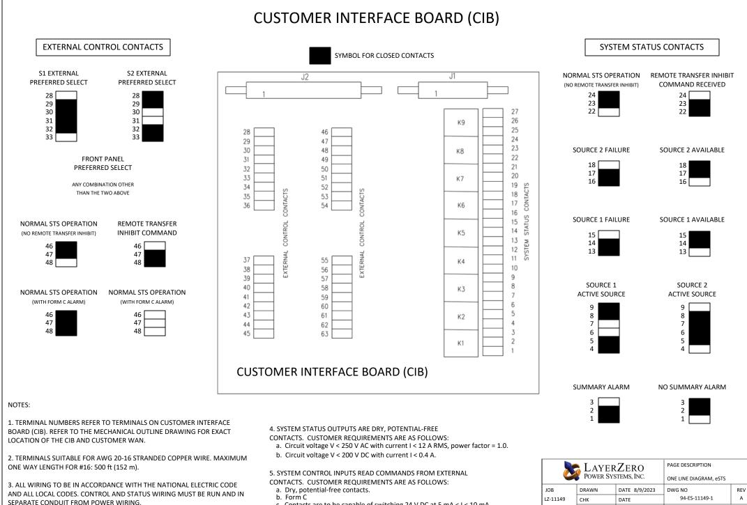
c. Contacts are to be capable of switching 24 V DC at 5 mA < I < 10 mA.
